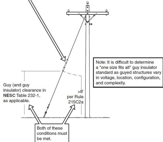
Fig. 215-5. Example of the use of insulators in anchor guys (Rules 215C2a, 232, and 279A).
